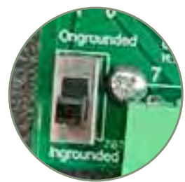
Choice of console-mounted micro-switch installation
