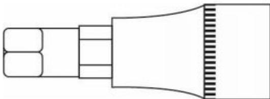
**Libellé article** DOUILLE EMBOUT HEXAGONAL 7mm L.55mm 1/2"
