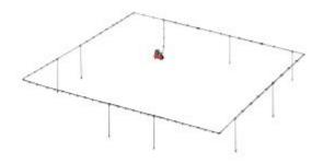
Item name ALUMINUM AIR PIPE AND FITTING KIT Ø32mm L.60m 8 DOWNPIPES
