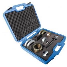
Item name WHEEL HUB BEARING TOOL SET HUB 2.1 Ø85mm
